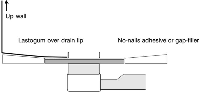
The slotted blue gasket membrane in the drain box is treated in the same manner as the tapes and corners in the Lastogum box; all are sandwiched between 2 coats of the Lastogum paste.
